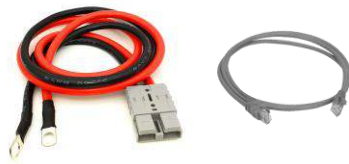
Model: RW-M5.3-PCable Details: Pair of 4AWG DC power cable (with M8 copper terminals) and RJ45 communication cable connect with hybrid inverter. The cable length can be customized based on customer requirements, default length is 1500mm.
